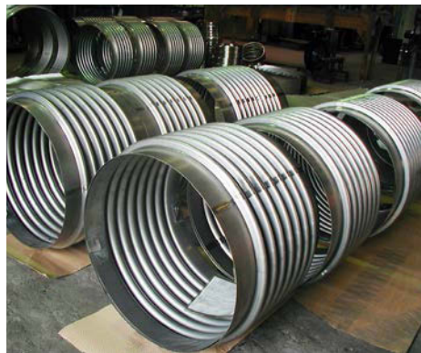
Bellows are subject to high bending stress well into the plastic range to achieve the movements required in FCC service.
