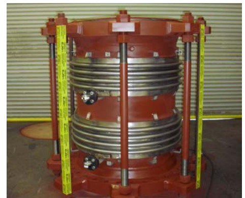
Two-ply dry nitrogen pressure thrust test ports installed between plies.
