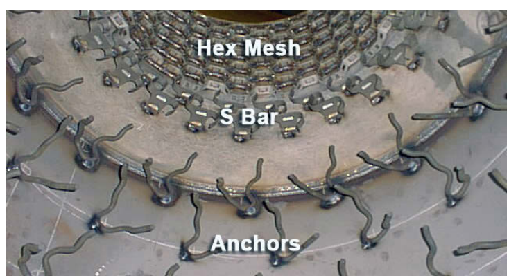
Hexmesh, S bar and anchors are used to secure the refractory inside lined expansion joints.
