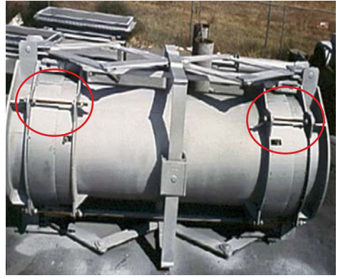
Control rods and telescopic covers can be seen on this FCCU expansion joints.
