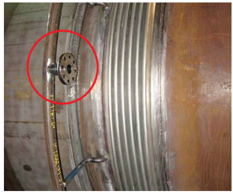
Typically numerous nozzles are used to introduce the purge equally around the annulus.
