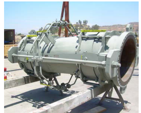
36" inside diameter universal hinged hot wall expansion joint for a reactor vapor line.
