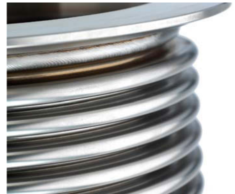
The finished bellows should be uniform in shape and pitch with no forming scratches or heavy tooling marks.
