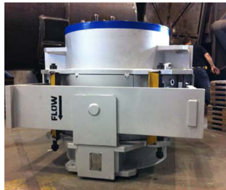
42" inside diameter FCCU Cold Wall Gimbal Expansion Joint.
